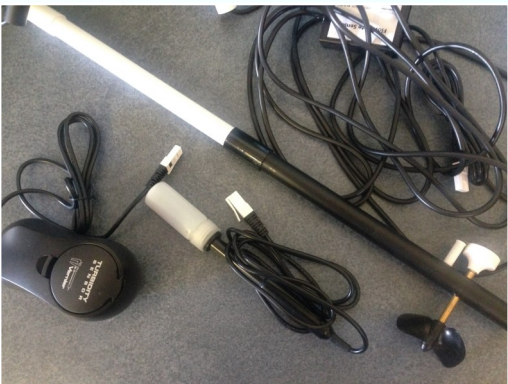
A new platform that was built for CreekWatch volunteers to collect water samples (above). A turbidity sensor, a dissolved oxygen probe and a flow-rate sensor (below).
